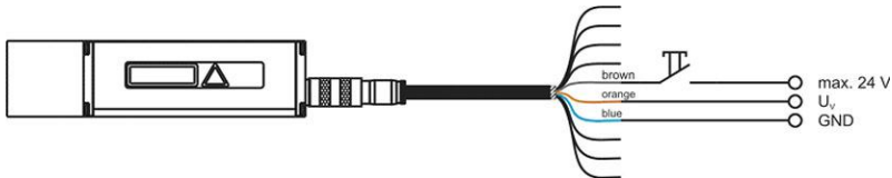
Figure 21: Wiring diagram of trigger input
