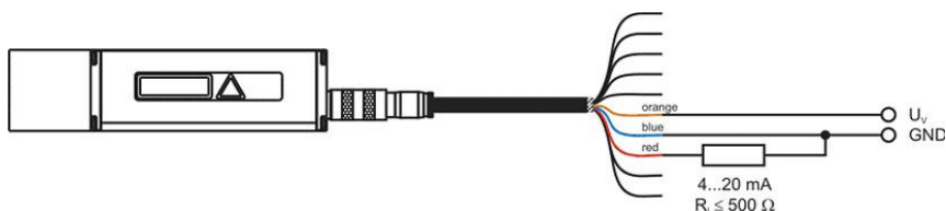
Figure 19: Wiring diagram of analog output
